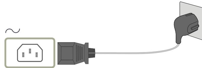
To use the product, connect the power cable to a power outlet and the
