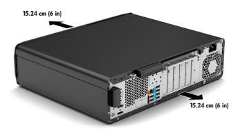
Be sure that the ambient air temperature is within specified limits. To locate specifications for your computer, see <u>Product specifications on page 10</u>.  For cabinet installation, ensure adequate cabinet ventilation and be sure that the ambient temperature within the cabinet does not exceed specified limits.
