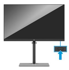
NOTE: If pressing the power button has no effect, the Power Button Lockout feature might be enabled. To disable this feature, press and hold the monitor power button for 10 seconds.
