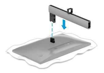
3. Attach the base to the monitor stand (1), and then tighten the screws (2).
