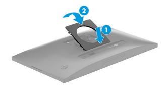
3. Remove the four screws from the VESA holes located on the rear of the monitor head (1), and then remove the monitor stand connector (2).
